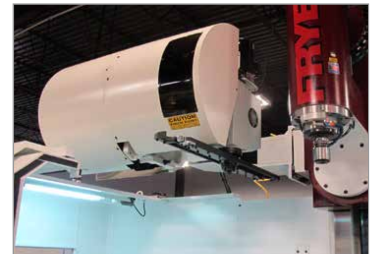
TOOL CHANGE POSITION ATC automatically moves in to allow fast tool changes. 40-tool capacity.
