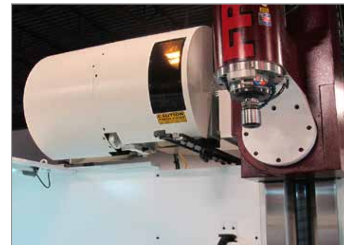
RETRACTED POSITION Allow for full movement of the head right or left +/- 110°.
