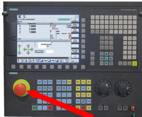
EMERGENCY STOP (E-STOP) BUTTON
