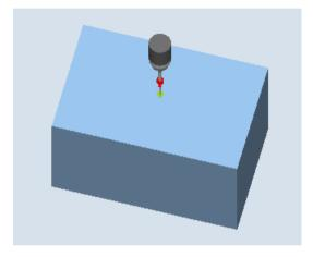
Image 3-7 Calibrate: Length at edge (CYCLE976)
