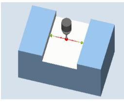
The measured difference of the groove width is used as basic variable for a tool offset, the position of groove zero point, as basis of a work offset.
