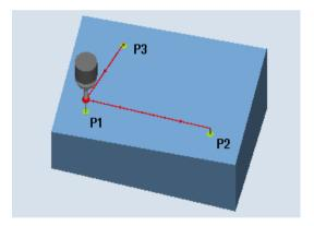
Image 3-17 Measure: Align plane (CYCLE998)
