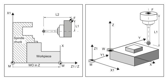
The position of tool reference point F in the machine coordinate system is defined with machine zero M as the **machine actual value**.
