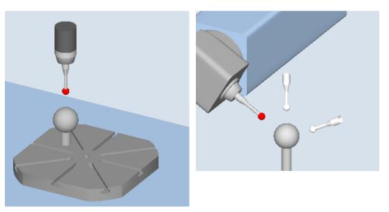
Measure: Kinematic (CYCLE996), 1st measurement, swivel table
