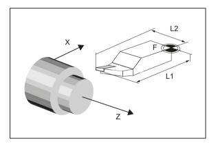
Image 2-3 Example: Lathe with G18
