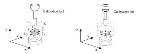
Image 3-31 Tool probe, disk and cube version
