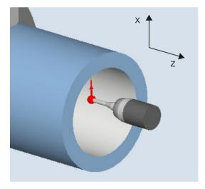
Image 3-4 Measure: Inside diameter (CYCLE974)
