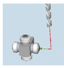
Image 3-26 Measure: drill (CYCLE982), example , tool position: ↓ radial position
