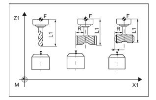
Image 3-35 Length measurement with and without offset
