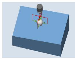
Measure: Sphere (CYCLE997), Example of "paraxial" positioning
