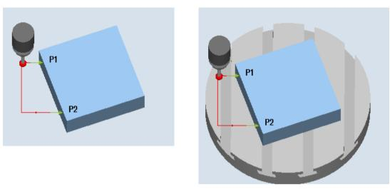
Measure: Align edge (CYCLE998), workpiece Measure: Align edge (CYCLE998), workpiece clamped on rotary table C axis
