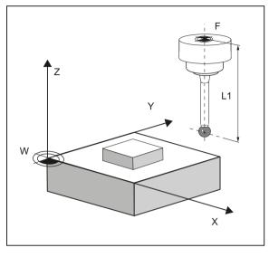
Image 2-2 Example: Milling machine with G17
