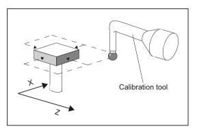
A probe must be calibrated before it can be used. To do this, when using measuring cycles in the AUTOMATIC mode, **before** calibration, the approximate values must be entered into the setting data listed above for the corresponding probe. Only then can the approximate position of the probe be identified in the measuring cycle.
