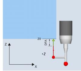
Measure: Edge (CYCLE978) measuring direction: -X
