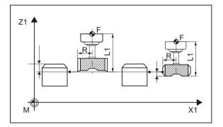
Image 3-41 Radius measurement with and without offset
