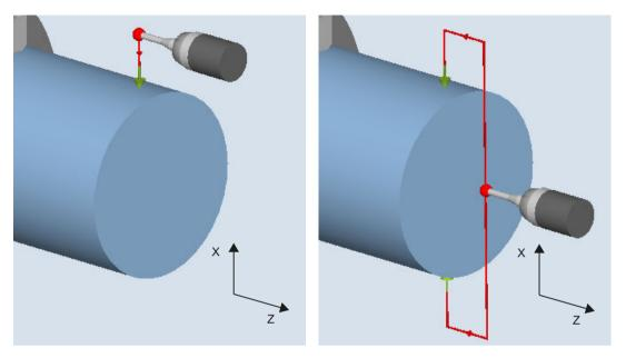
Measure: Outside diameter (CYCLE974) with/ Measure: Outside diameter (CYCLE994) without reversal of the workpiece above and below the turning center
