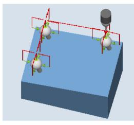
Measure: 3 balls (CYCLE997), Example of "paraxial positioning"
