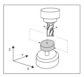
Image 2-5 Measuring a milling cutter
