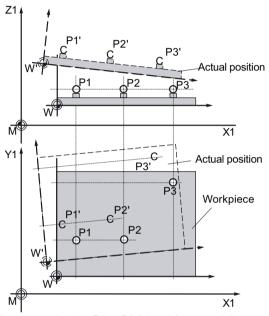
3 connected points P1 to P3 (triangle) are spatially offset, and can be arranged, rotated: P1', P2', P3'
