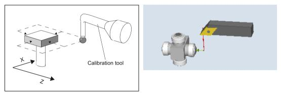
Calibrating the tool probe with a calibration toolCalibrating a tool probe with a turning tool
