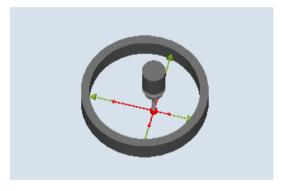
Image 3-8 Calibrate: Radius in ring (CYCLE976)
