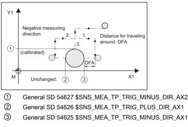
Image 3-30 Calibrate probe (CYCLE971) with offset axis, example G17: Determine center in X, calibrate in Y
