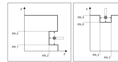
Geometry of the calibration groove, example G18, SL=7
