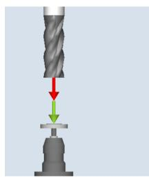
Measure: Milling tool (CYCLE971), example, length
