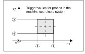
Image 3-19 Tool probe, machine-related (G18)
