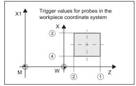
Image 3-20 Tool probe, workpiece-related (G18)
