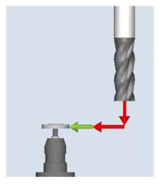
Measure: Drilling tool (CYCLE971), example, radius
