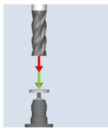
Measure: Drilling tool (CYCLE971), example, length
