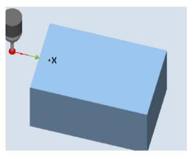
Calibrate: Radius at edge (CYCLE976), calibration direction
