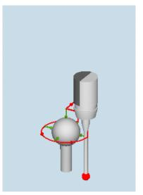
Measure: Angular deviation, spindle (CY-CLE995), 2nd measurement
