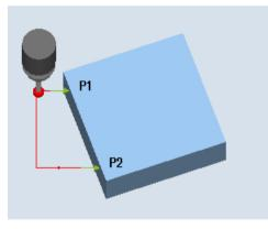
Image 3-12 Aligning the edge (CYCLE998), intermediate positioning "parallel to the axis"
