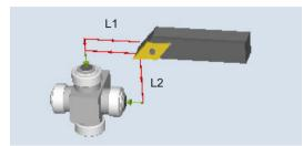
Image 3-22 Measure: Turning tool (CYCLE982), example: Complete measuring
