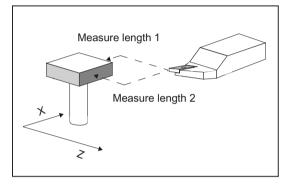
Image 2-7 Measuring a turning tool
