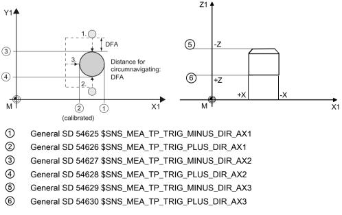
Image 3-32 Determining the probe center in the 2nd axis of the plane, calibration +X
