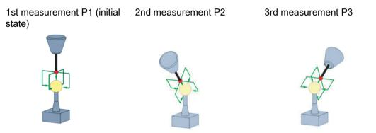
With the 2nd and 3rd measurements, the rotary axis to be measured is rotated around the largest possible angle. The calibration ball position must be stationary during the measurements.
