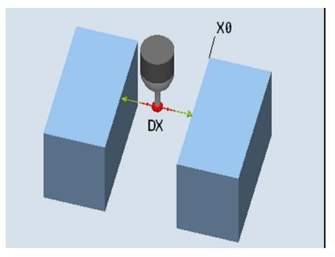
Image 3-9 Calibrate: Radius between 2 edges (CYCLE976)
