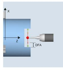
Calibrate: Probe in groove (CYCLE973), example G18, SL=7
