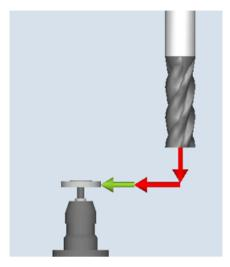
Measure: Milling tool (CYCLE971), example, radius
