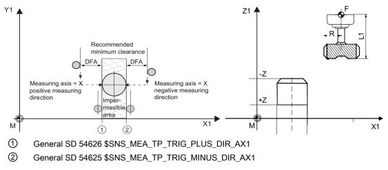
Image 3-37 Calibrate probe (CYCLE971), starting positions for calibration in the plane
