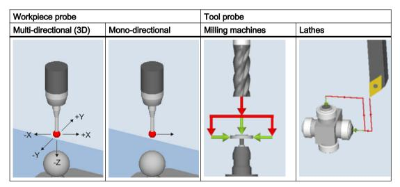
The probes also differ in the form of the stylus tip:
