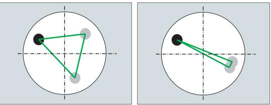
The calculated inside angle of the rotary axis angle segment is monitored in the **TVL** parameter. Angle values of < 20 degrees can cause inaccuracies when calculating the kinematics.
