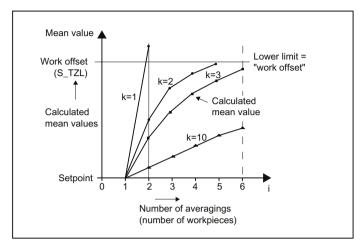
Computational characteristic of the mean value with different weightings k
