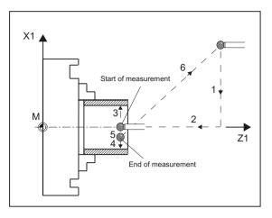
Image 3-5 Positions of the probe when measuring the inner diameter using 2-point measurement (CYCLE994)
