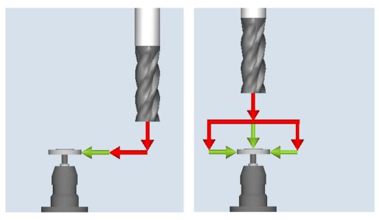
Calibrate: Probe (CYCLE971), axis-by-axis
