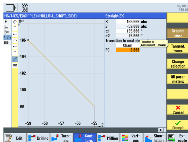
Figure 9-18 Specifying the inclined straight line contour
