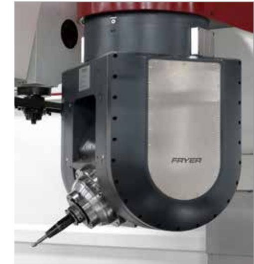
The Kessler heavy duty head is designed for steel and tough alloy machining.
