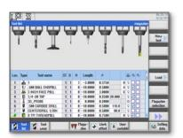
The tool management page stores your tool information in a graphical format. In addition, tools can be given tool numbers or actual names like .500 drill or .375 CBD end mill. Each tool can be managed for wear and switched automatically when the tool run time is reached.
