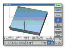
The standard part probe cycles use a simple GUI to make part set-up simple. The cycles include edge find, part skew, pocket, boss and many more. The cycles can also be used to measure the part and display dimensions on the screen, much like a CMM.
