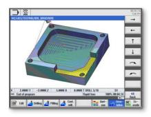
After the part is programmed it can be simulated to show the operations and tool paths. Simulation will also work with programs brought in from a CAM system that were output in G code. Cycle time is displayed also.
