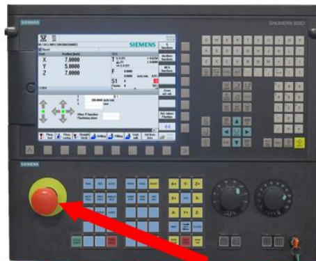
EMERGENCY STOP (E-STOP) BUTTON
