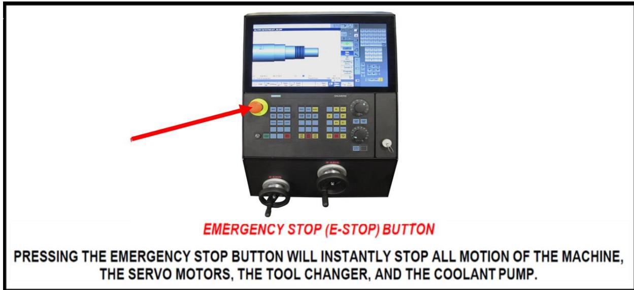
1. Use the emergency stop button to stop all machine motion in the event of an emergency.
