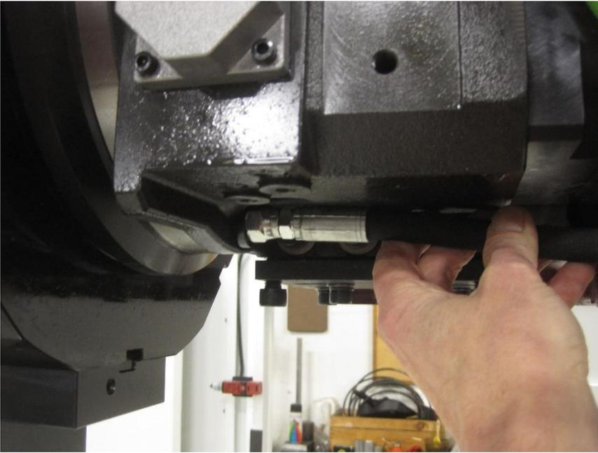
5. Install Eyehook, and chock strap around the faceplate neck, to support the turret with overhead crane, or forklift. Loosen the 8 turret mounting bolts, and remove.
