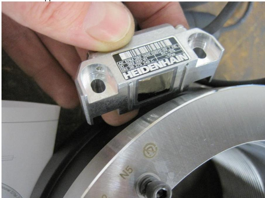
You can cut a .0059" plastic shim , 1/2" wide x 5" long, hold the reader head tight on the ring with the shim in between, tighten the screws, then pull shim out.
