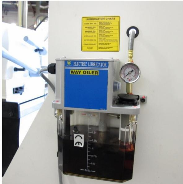
when the spindle and axes are moving. If there is no machine movement the pump will not pump unnecessary oil. This method greatly reduces way lube usage and keeps oil out of the machine coolant sump and prevents fouling.
