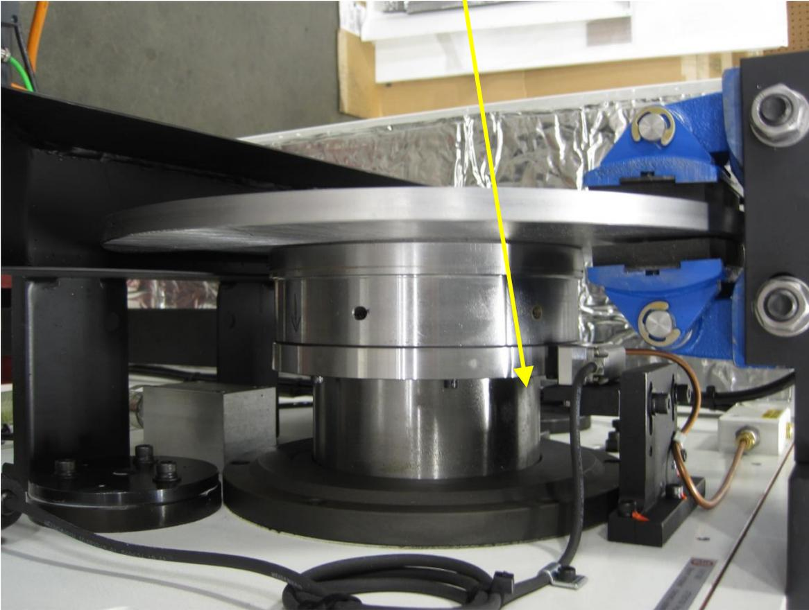
Check the Heidenhain reader head for damage, if not damaged, reset the spacing to .0059" See the HH book that was shipped with the machine in the Folder in the electrical cabinet.
