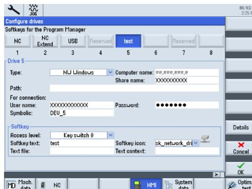
8. Press the **OK** key. The entries are checked. A window with the appropriate message opens if the data is incomplete or incorrect. Acknowledge the message with **OK** key. If you press the **CANCEL** key, then all of the data that has not been activated is rejected.
