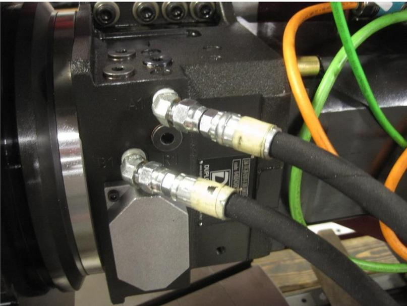
4. Remove Coolant hose (Jic 6) and cap off.
