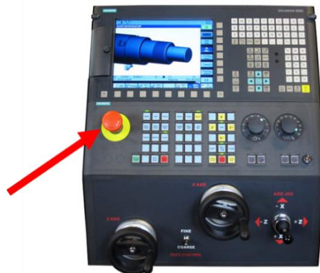
EMERGENCY STOP (E-STOP) BUTTON
