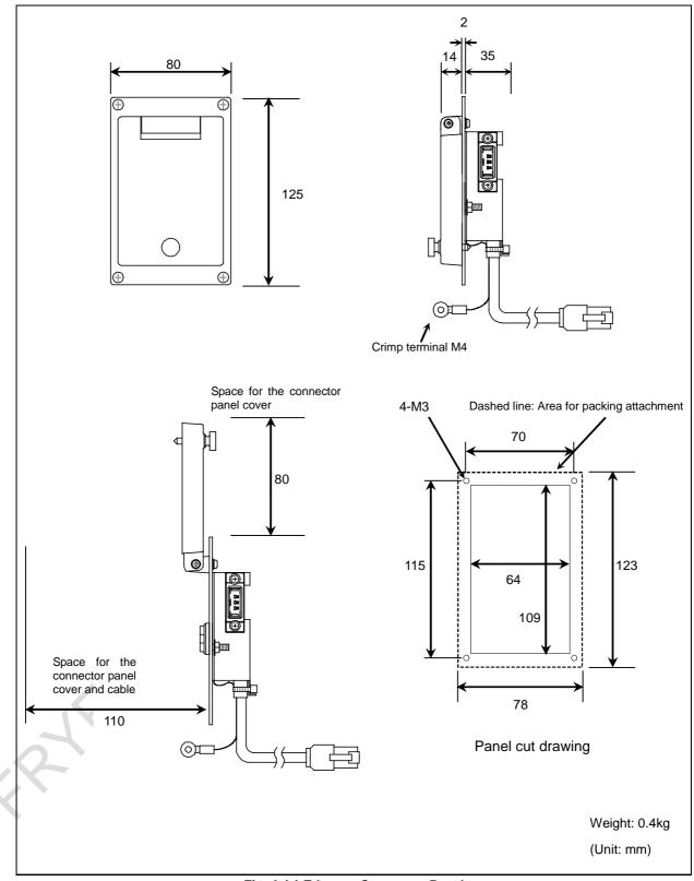
Fig. A (s) Ethernet Connector Panel
