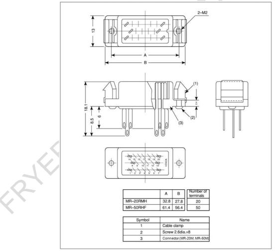
Fig. A (ah) Connector (male) manufactured by HONDA TSUSHIN KOGYO
