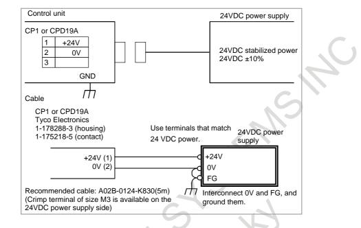
Supply the power to the control unit from a 24 VDC power supply.
