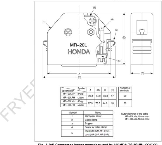
Fig. A (af) Connector (case) manufactured by HONDA TSUSHIN KOGYO
