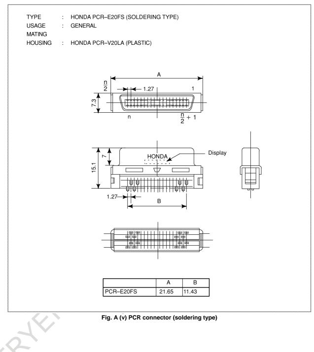
Fig. A (v) PCR connector (soldering type)
