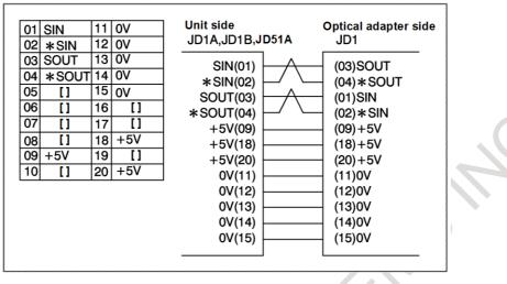
Recommended wire material A66L-0001-0284#10P (#28AWG × 10 pairs)
