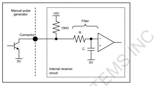
The points (thresholds) at which the input signal to the receiver changes are: 3.7 V or higher when the input signal state changes from the low level to the high level 1.5 V or lower when the input signal state changes from the high level to the low level
