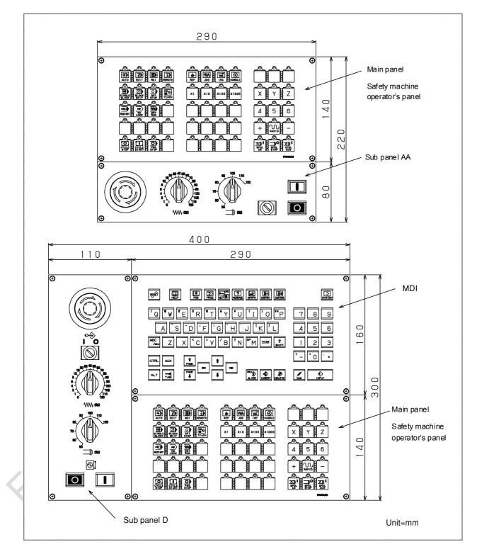
The following figure is the example of composition when using the safety machine operator's panel type B.
