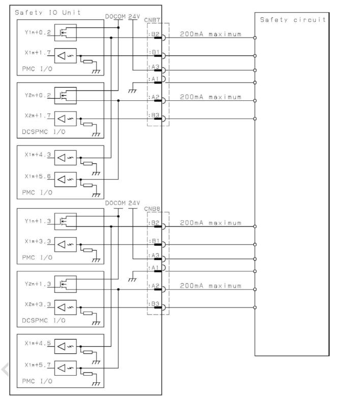
Duplicated input and output signals are connected to Safety IO Unit as PMC I/O and DCSPMC I/O.
