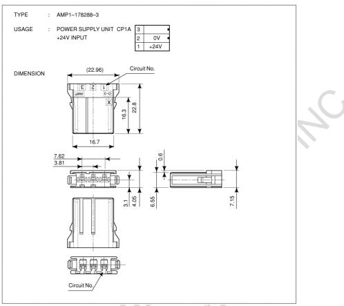
Fig. A (ac) Connector (3) for +24 V power supply manufactured by Tyco Electronics
