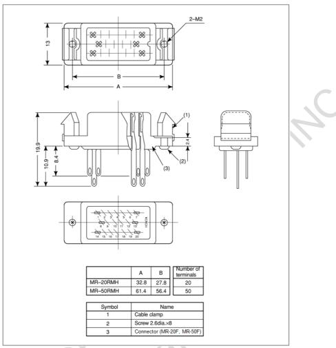
Fig. A (ai) Connector (female) manufactured by HONDA TSUSHIN KOGYO
