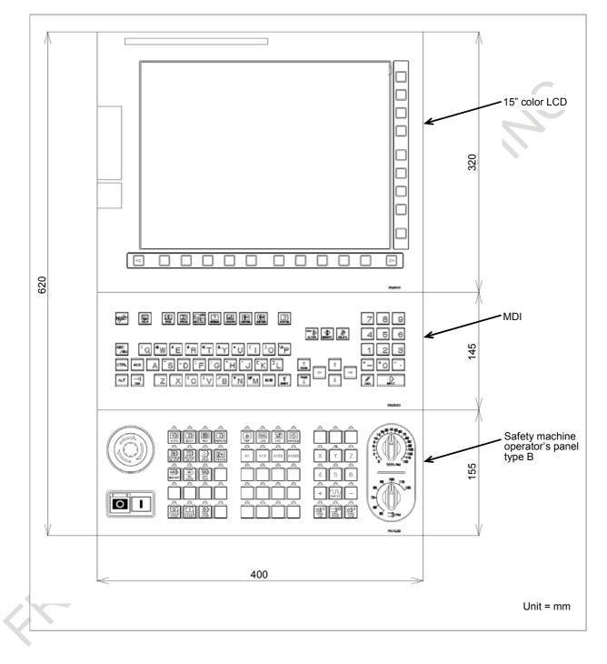
The following figure is the example of composition when using the safety machine operator's panel -BK10.
