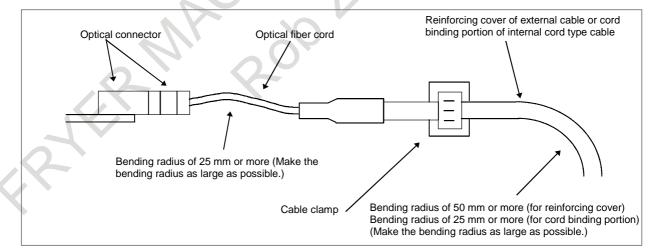
Fig. D (e) Fixing the optical fiber cable with a clamp
