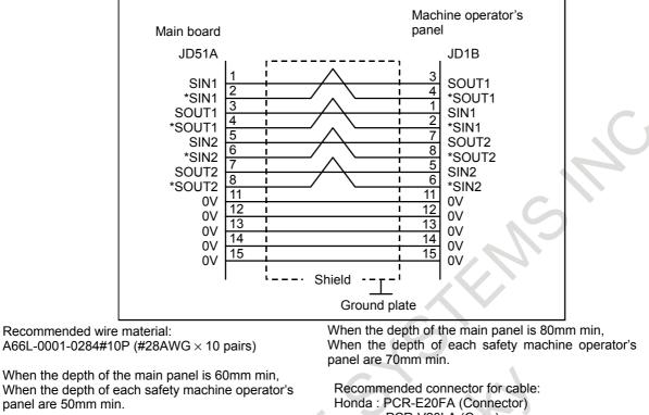
Recommended connector for cable: Hirose electric FI30-20S (Connector) FI-20-CV7 (Case) Recommended connector for cable: Honda : PCR-E20FA (Connector) PCR-V20LA (Case) Hirose electric : F130-20S (Connector) F1-20-CV2 (Case) Fujitsu : FCN-247J020-G/E (Connector) FCN-240C020-Y/S (Case) Molex : 52622-2011 (Connector) 52624-2015 (Case)
