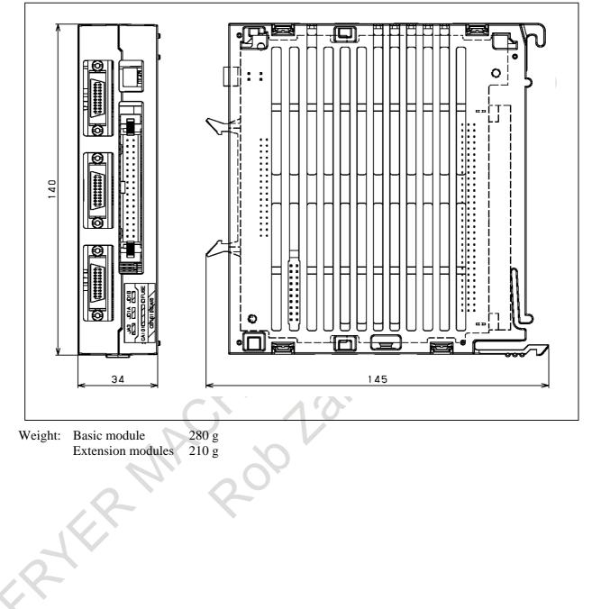
The basic module and extension modules have the same dimensions.
