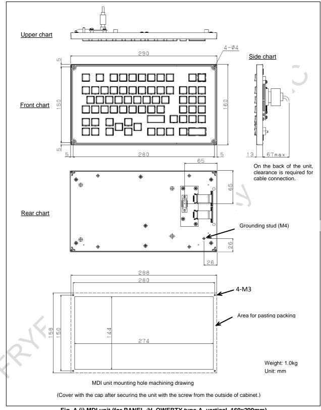
Fig. A (i) MDI unit (for PANEL *i*H, QWERTY type A, vertical, 160x290mm)
