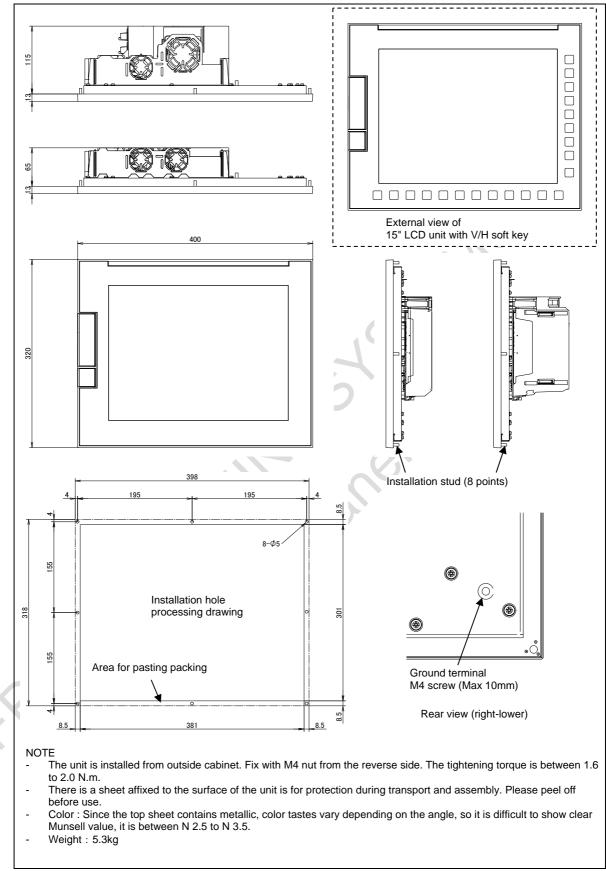
Fig. A (e) LCD-mounted type control unit - 15" LCD unit \* for PANEL iH
