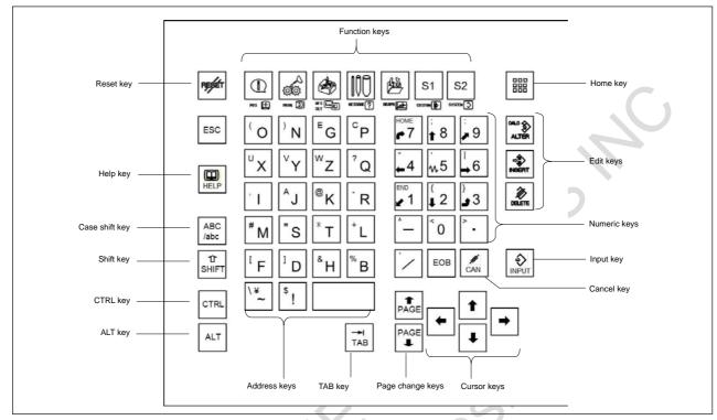
MDI unit (for PANEL *i*H, with machining center system (M series), ONG, horizontal, 220x230mm)
