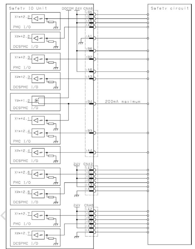
Duplicated input and output signals are connected to Safety IO Unit as PMC I/O and DCSPMC I/O.
