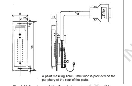
Fig. A (r) Punch panel (for Stand-alone type control unit)
