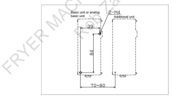
When using both a basic unit (or analog basic unit) and additional unit, install the units as shown above, with the mounting holes horizontally separated by 70 to 80 mm.
