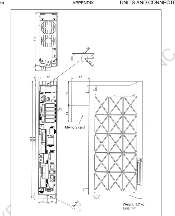
Fig. A (f) LCD-mounted type control unit – 2slots
