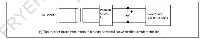
Fig. 4.1.2 (b) Example of a power supply circuit that cannot maintain 24 VDC
