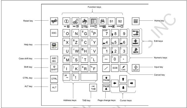
MDI unit (for PANEL *i*H, with lathe system (T series), ONG, horizontal, 220x230mm)
