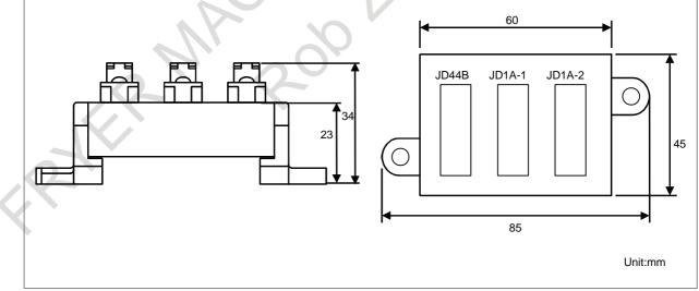
Allow a clearance of about 10 cm above the adapter for connection and routing of cables.
