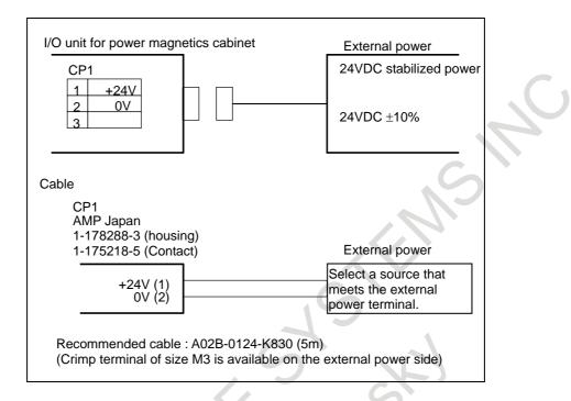
Supply power to the I/O unit for power magnetics cabinet from external power.
