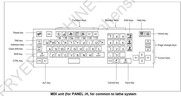
(T series)/machining center system (M series), QWERTY type B, vertical, 145x400mm)
