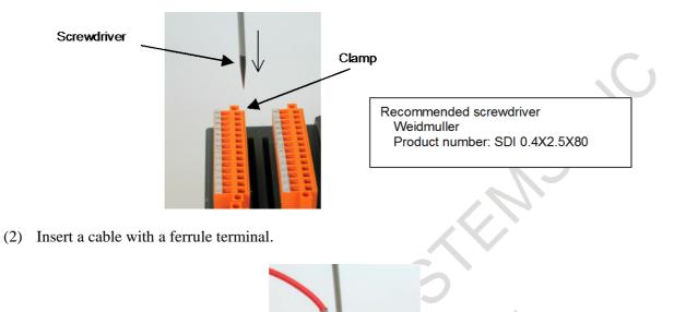
(3) Extract the screwdriver from the clamp to complete cabling.
