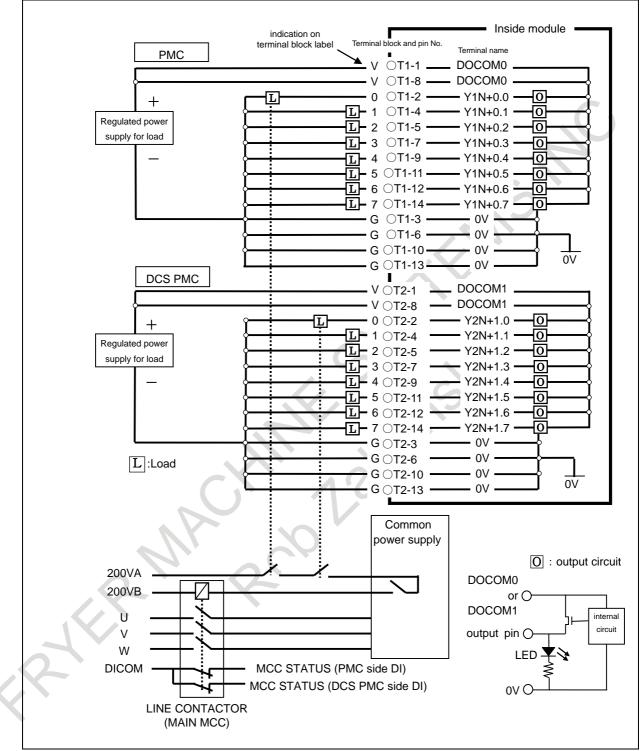
Fig. 8.6.5.4(h) DO connection of basic module (DCS-enabled version)
