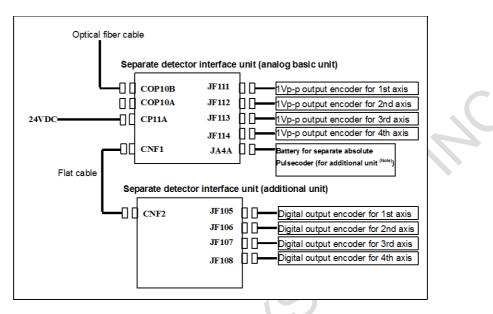
(4) When encoders with an analog output of 1 Vp-p are connected to the 1st to 4th axes and digital output encoders are connected to the 5th to 8th axes
