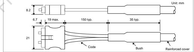
Fig. D (b) External dimensions of external cable
