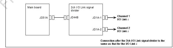
Specification of the 2ch I/O Link signal divider: A20B-1007-0680 (Weight: 60g)
