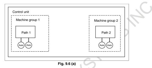
To prevent an emergency stop in one machine group from affecting another within a multi-path control system, a separate emergency stop circuit (see Fig. 9.6 (b)) must be provided for each machine group.
