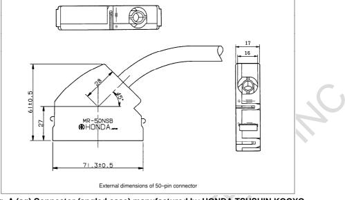
Fig. A (ag) Connector (angled case) manufactured by HONDA TSUSHIN KOGYO
