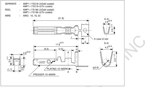
Fig. A (ae) Contact for connector manufactured by Tyco Electronics
