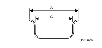
External dimensions of a recommended DIN rail
