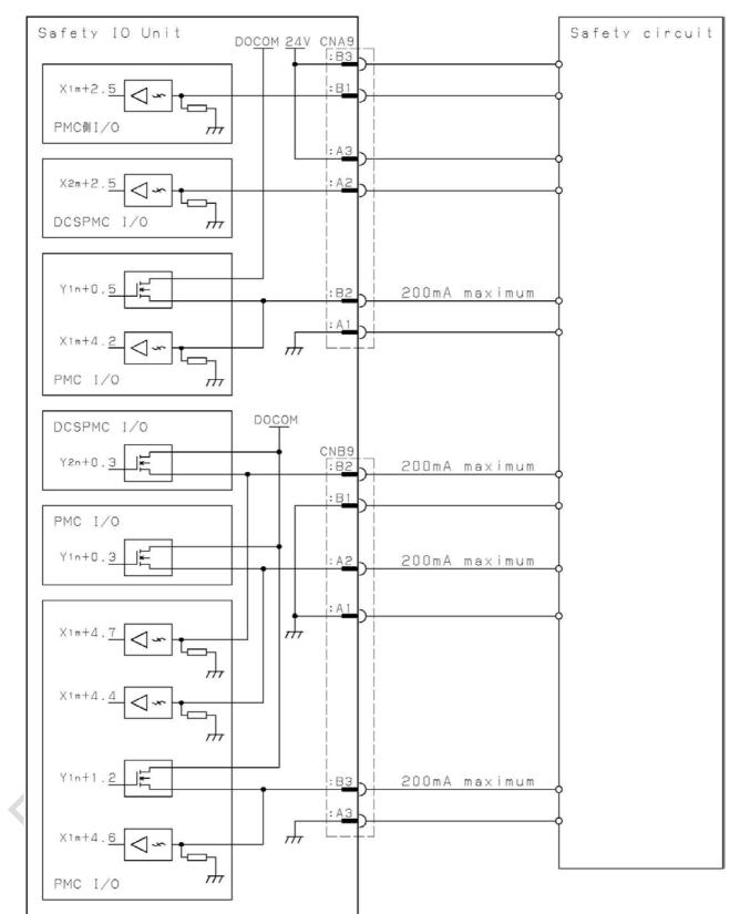
Duplicated input and output signals are connected to Safety IO Unit as PMC I/O and DCSPMC I/O.
