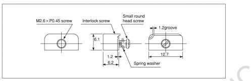
Fig. A (ap) Locking plate for reader/punch interface connector
