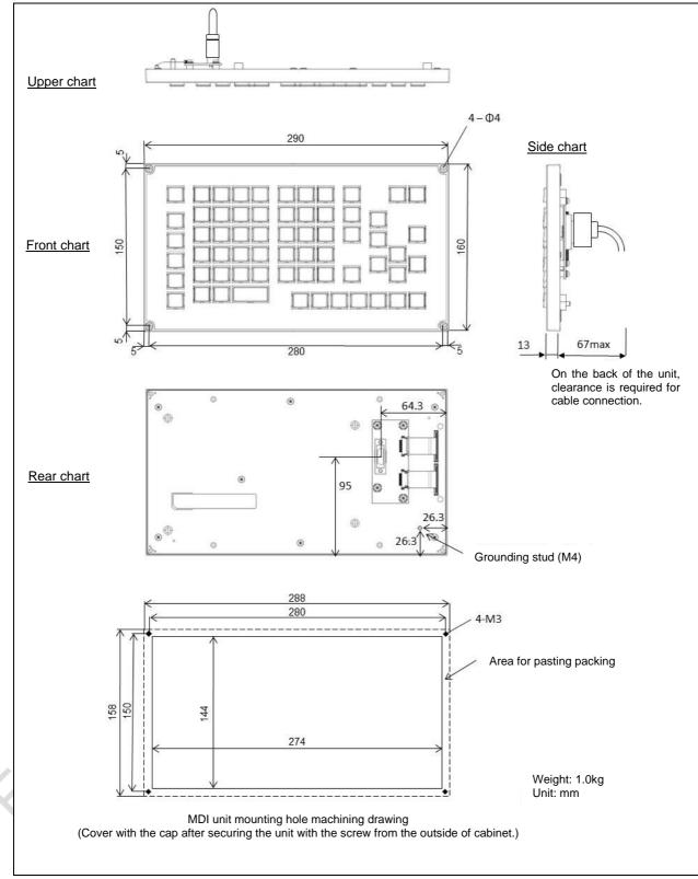
Fig. A (h) MDI unit (for PANEL *i*H, ONG, vertical, 160x290mm)
