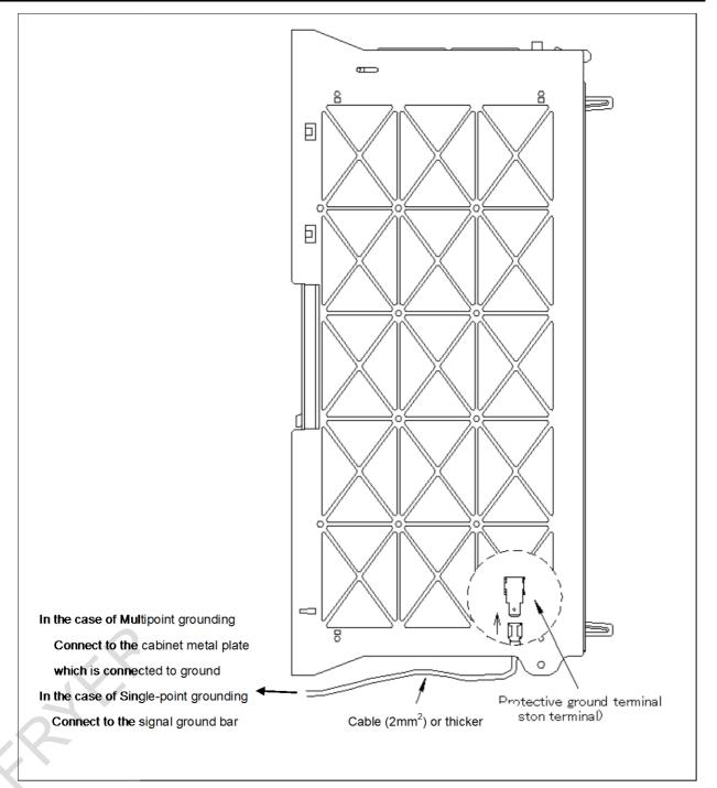
Connect the 0V line of this unit to the cabinet's metal plate which is connected to ground or signal ground bar nearby via the protective ground terminal. Ground cable can be connected to the terminal from the bottlom of the unit case. Refer to Item 3.4.1.1 about Multipoint grounding or Single-point grounding. Use a faston terminal for series 250 as cable terminal.
