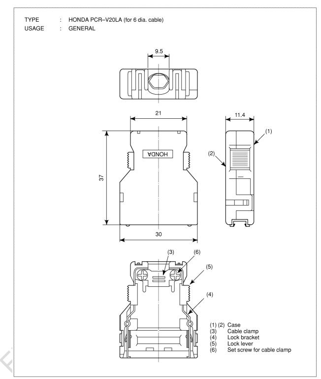
Fig. A (x) Connector case (PCR type manufactured by HONDA TSUSHIN KOGYO)
