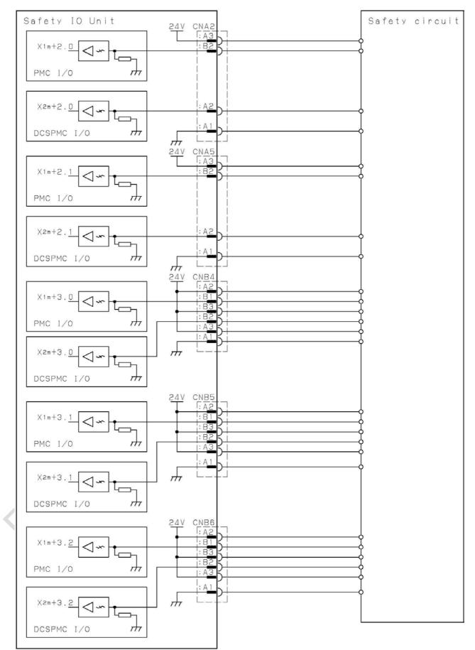
Duplicated input and output signals are connected to Safety IO Unit as PMC I/O and DCSPMC I/O.
