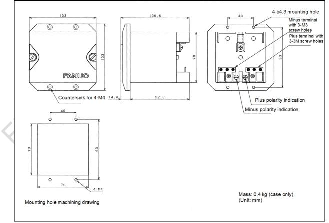
Fig. A (o) Battery case for separate absolute pulse coder
