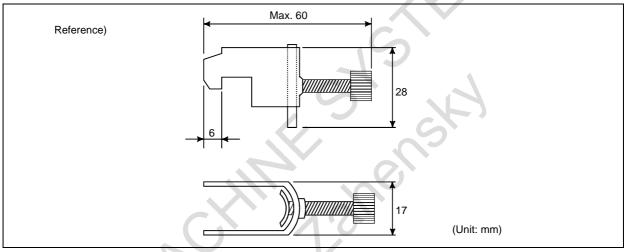
Fig. 3.4.6 (e) Clamping metal fixture (outline drawing)
