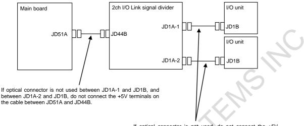
If optical connector is not used, do not connect the +5V terminals of the cable between JD1A-1(JD1A-2) and JD1B.
