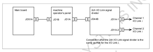
Connection between the main board and machine operator's panel
