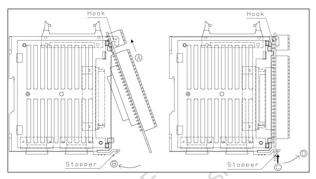
Method of install to I/O MODULE FOR CONNECTOR PANEL is as follows.
