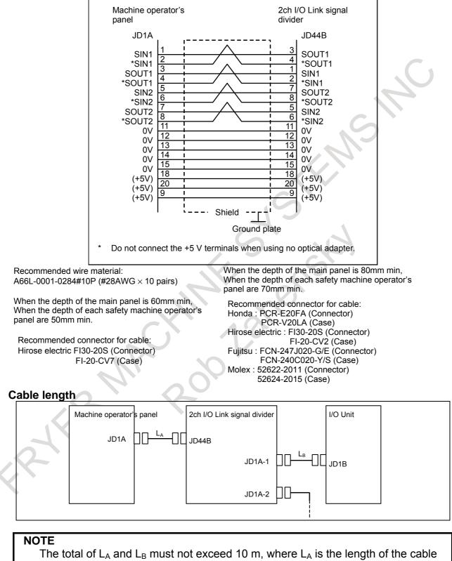
Ine total of  $L_A$  and  $L_B$  must not exceed 10 m, where  $L_A$  is the length of the cable between connector JD1A on the machine operator's panel and connector JD44B on the 2ch I/O Link signal divider, and  $L_B$  is the length of the cable between connector JD1A-1 or JD1A-2 on the 2ch I/O Link signal divider and connector JD1B on the I/O unit. When all cables are laid within the same cabinet, however, a total cable length of up to 15 m is allowed.
