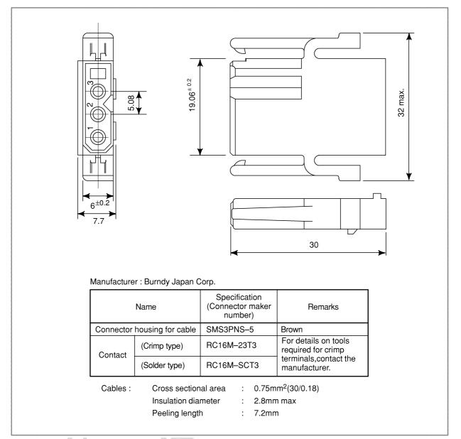
Fig. A (ak) Connector (3 pins/brown) manufactured by Burndy Japan
