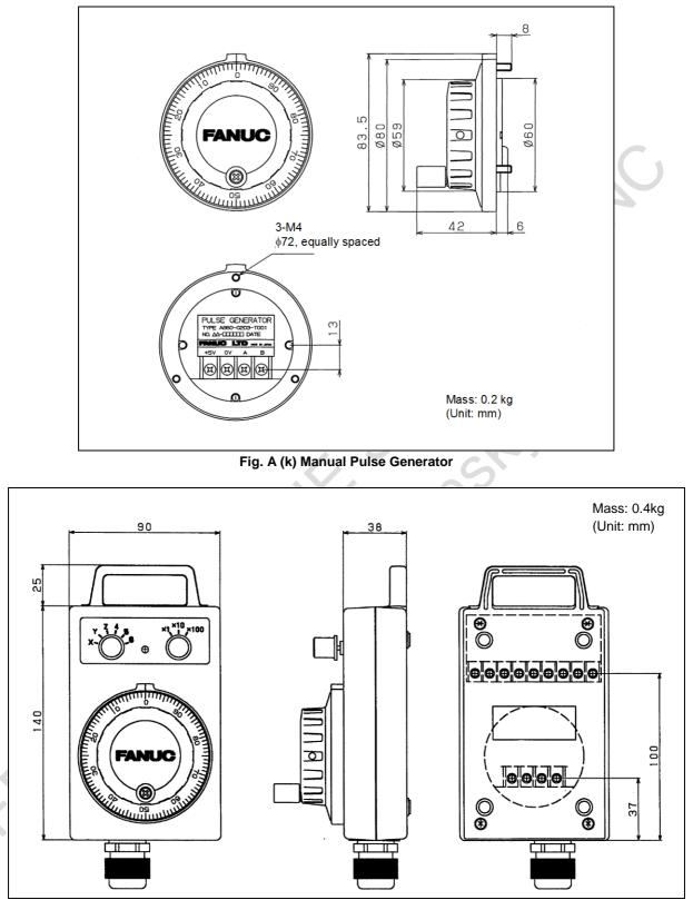
Fig. A (I) Pendant type Manual Pulse Generator
