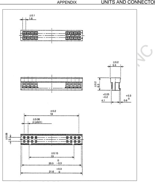
Fig. A (am) Connector (for MDI) manufactured by Japan Aviation Electronics
