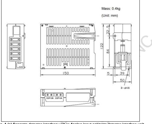
Fig. A (n) Separate detector interface unit or Analog input separate detector interface unit
