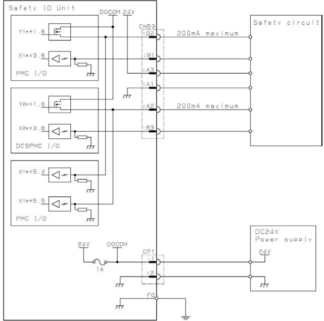
Duplicated input and output signals are connected to Safety IO Unit as PMC I/O and DCSPMC I/O.
