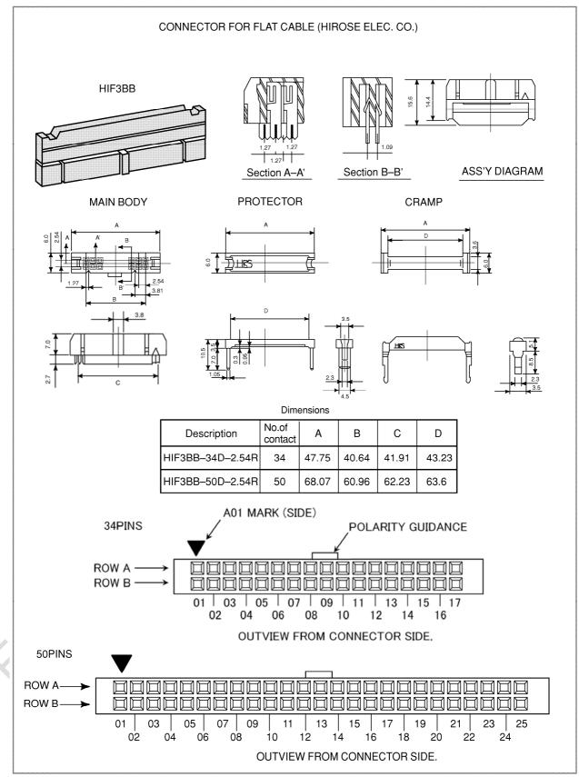
Fig. A (al) Connector for flat cable manufactured by HIROSE ELECTRIC
