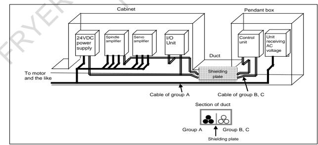
Fig. 3.4.4 Cable layout example
