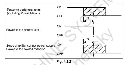
t4:500ms It is meant that the power of interest is turned off not earlier than 500 ms before the power to the control unit is turned off.
