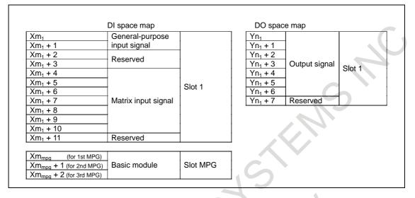
$Xm_1$ ,  $Xm_{mpg}$ , and  $Yn_1$  indicate the start address at allocation.
