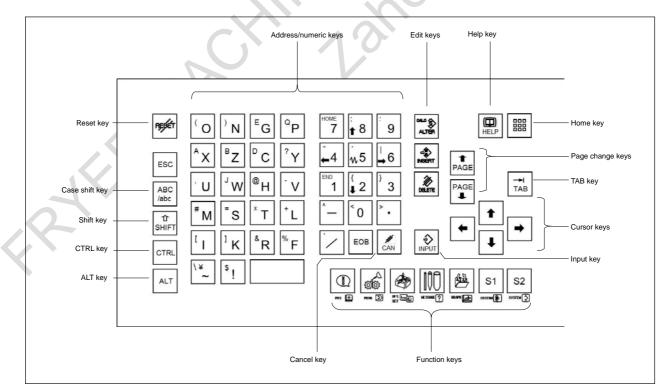
MDI unit (for PANEL *i*H, with lathe system (T series), ONG, vertical, 160x290mm)
