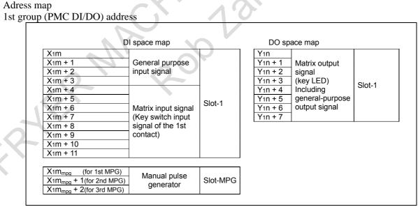
X1m, X1mmpg, and Y1n indicate the start address at allocation.
