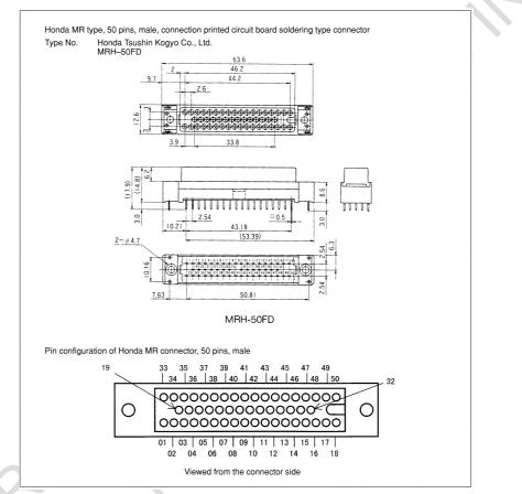
Fig. A (aq) Connector (for distribution I/O connection printed circuit board) manufactured by HONDA TSUSHIN KOGYO
