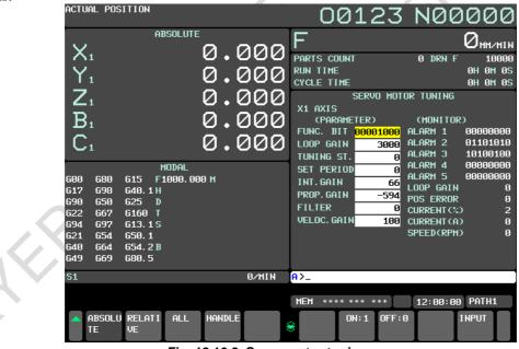
Fig. 12.16.2 Servo motor tuning screen
