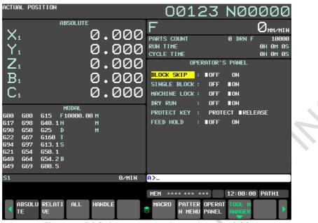
Fig. 12.20 (b) Software operator's panel screen (2/2)
