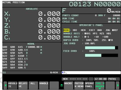
Fig. 12.20 (a) Software operator's panel screen (1/2)
