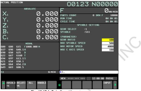
Fig. 12.17.1 Spindle setting screen
