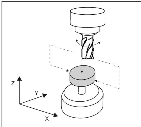
Image 2-5 Measuring a milling cutter
