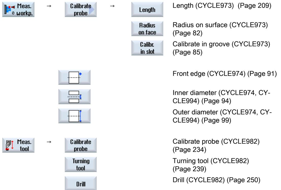
**Turning technology with extended milling technology menu tree**
