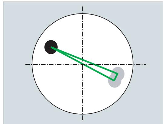
The calculated inside angle of the rotary axis angle segment is monitored in the **TVL** parameter. Angle values of < 20 degrees can cause inaccuracies when calculating the kinematics.
