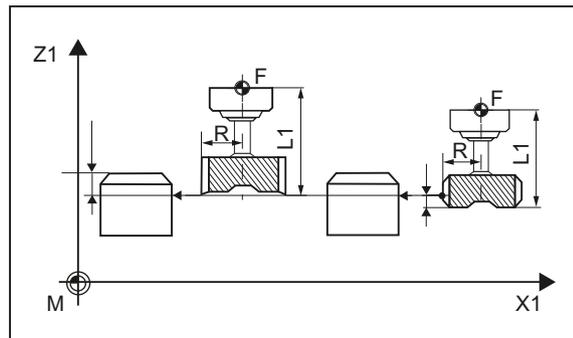
Image 3-36 Radius measurement with and without offset
