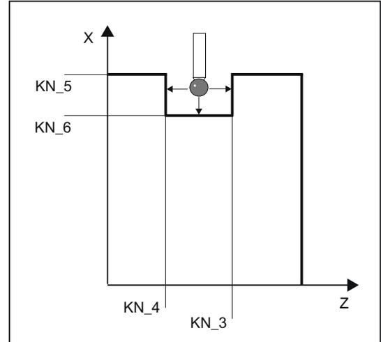
Geometry of the calibration groove,
