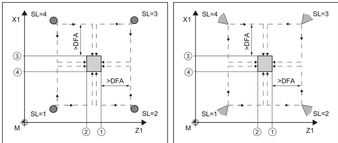
Cutting edge positions 1 to 4 and suitable approach positions for both axes (machine-related)
