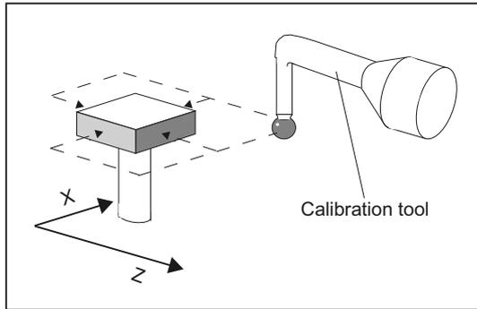
A probe must be calibrated before it can be used. To do this, when using measuring cycles in the AUTOMATIC mode, **before** calibration, the approximate values must be entered into the setting data listed above for the corresponding probe. Only then can the approximate position of the probe be identified in the measuring cycle.
