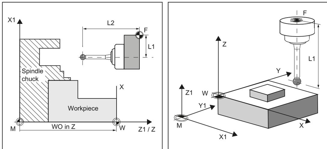
The position of tool reference point F in the machine coordinate system is defined with machine zero M as the **machine actual value**.
