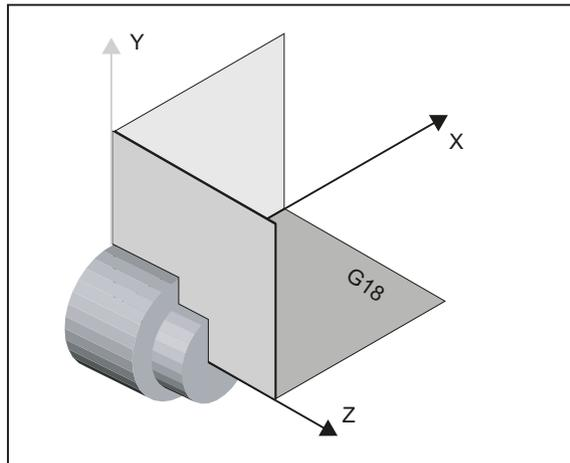
Turning machines generally only use axes Z and X and therefore:
