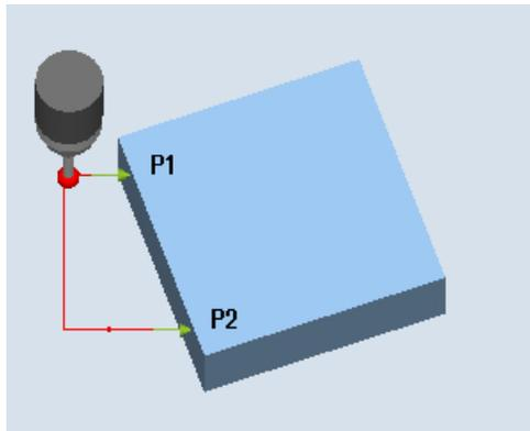
Measure: Align edge (CYCLE998), workpiece clamped in the plane
