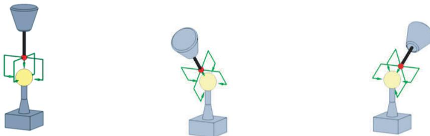
With the 2nd and 3rd measurements, the rotary axis to be measured is rotated around the largest possible angle. The calibration ball position must be stationary during the measurements.
