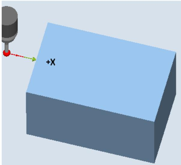
Image 2-8 Measurement operation sequence, example set edge (CYCLE978)
