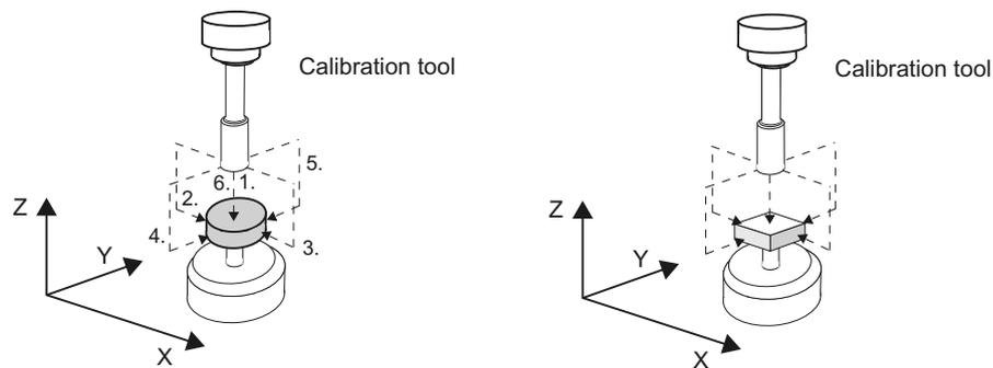
Image 3-31 Tool probe, disk and cube version
