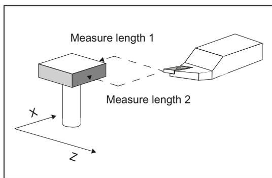
Image 2-7 Measuring a turning tool
