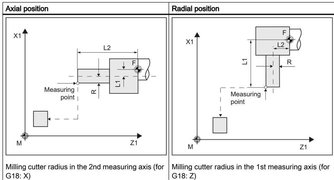
**Measurement with rotating/stationary spindle**
