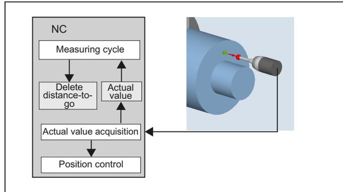
The principle of "flying measurement" is implemented in the SINUMERIK control. The probe signal is processed directly on the NC so that the delay when acquiring measured values is minimal. This permits a higher measuring speed for the prescribed measuring precision and time needed for measuring is reduced.
