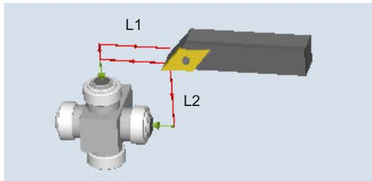
Image 3-22 Measure: Turning tool (CYCLE982), example: Complete measuring
