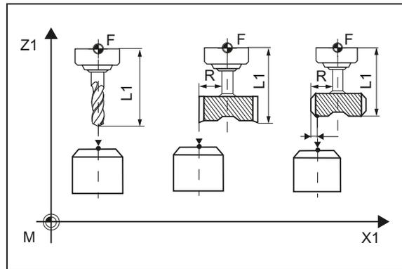
Image 3-35 Length measurement with and without offset
