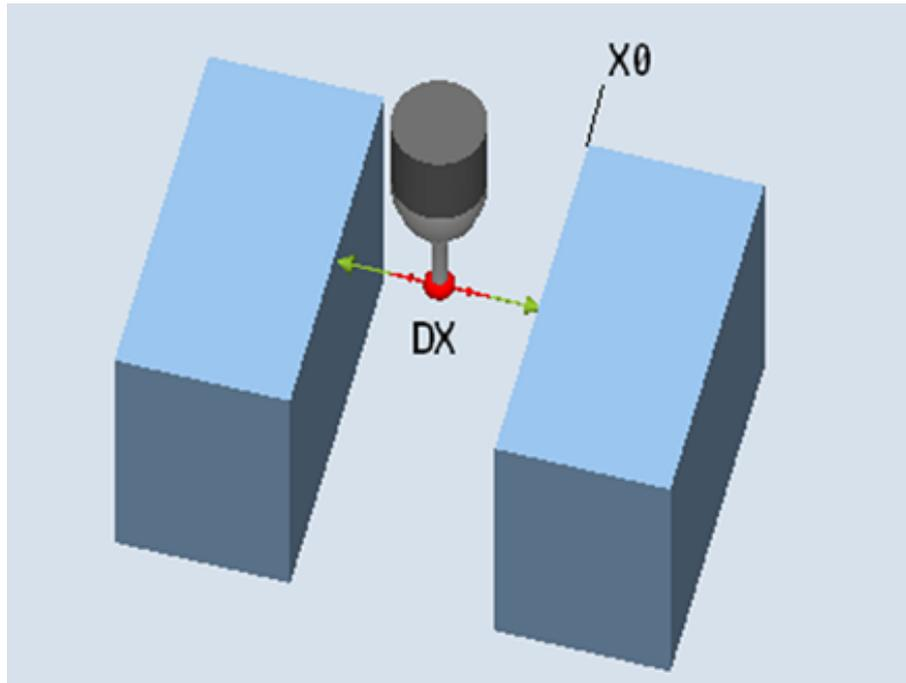
Image 3-9 Calibrate: Radius between 2 edges (CYCLE976)
