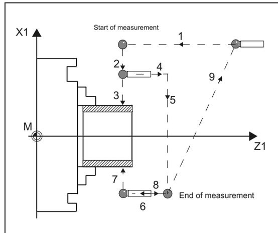
Image 3-6 Positions of the probe when measuring the outer diameter (CYCLE994) with retraction path in X and Z
