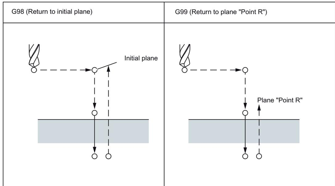
Figure 4-3 Plane for the return point (G98/G99)
