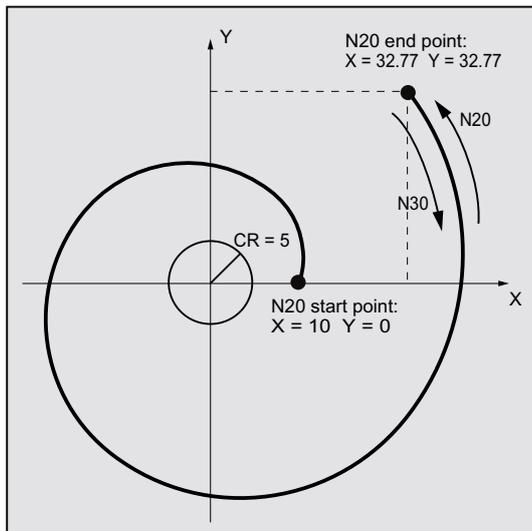
An involute can be traversed in space in case of additional specification of paths vertical to the active plane.
