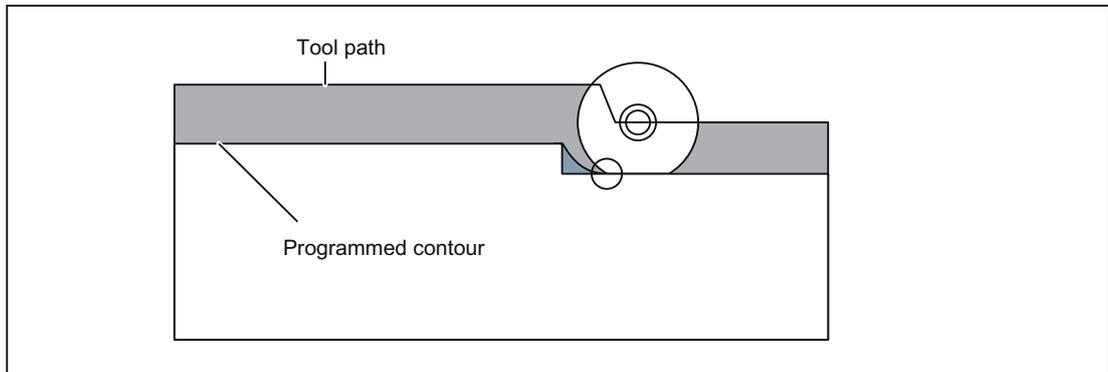
Figure 3-18 Contour definition shorter than tool radius
