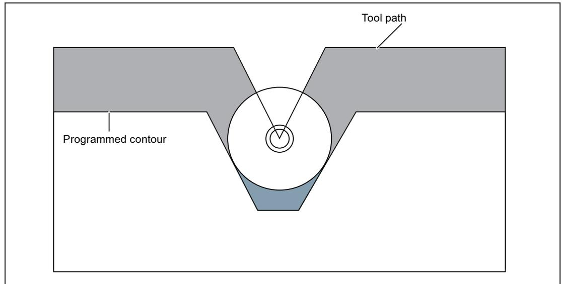
Figure 3-19 Tool radius too large for internal machining
