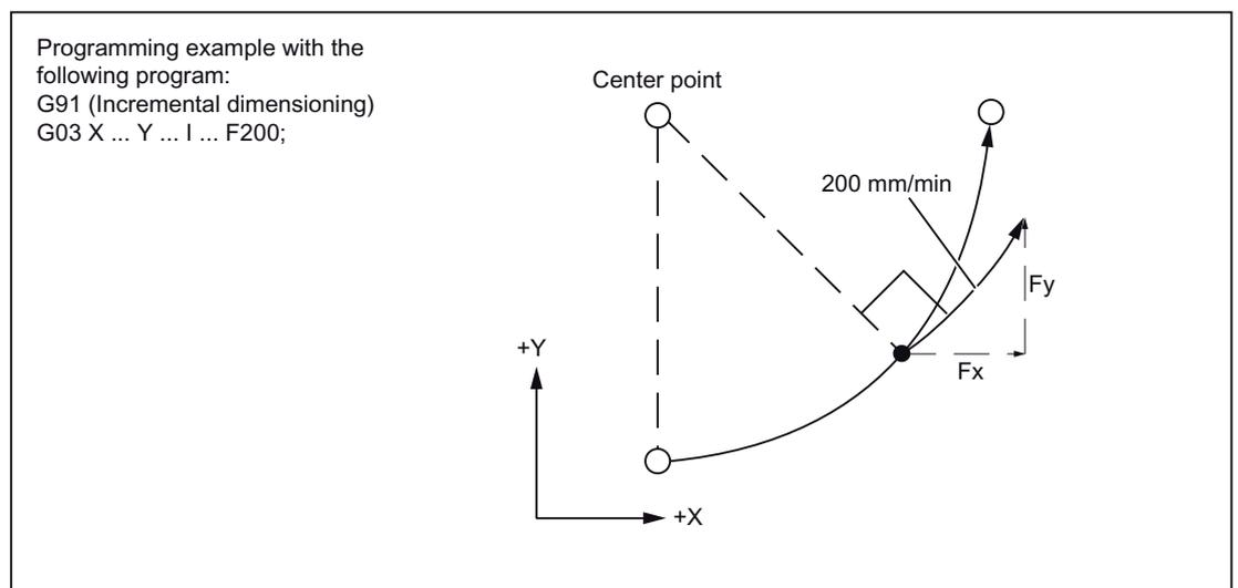
Figure 1-2 Circular interpolation with 2 axes
