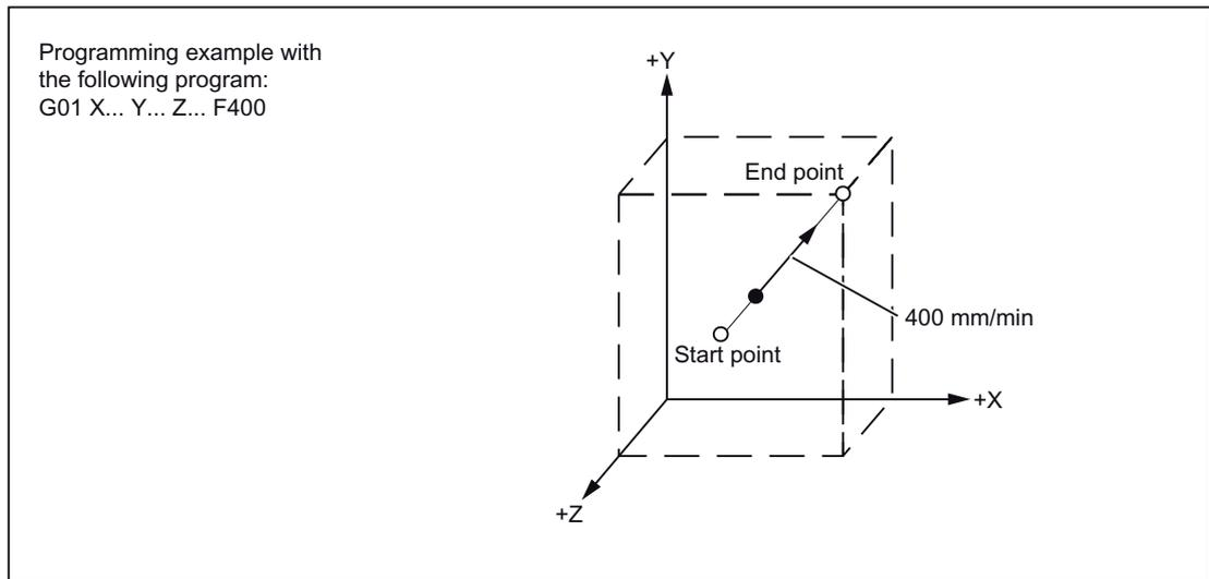
Figure 1-3 Feed in case of 3D interpolation
