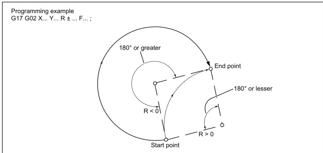
Figure 2-4 Circular interpolation with specification of Radius R
