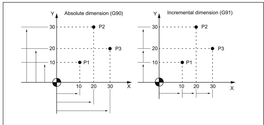
Figure 3-7 Absolute and incremental dimensioning (G90, G91)
