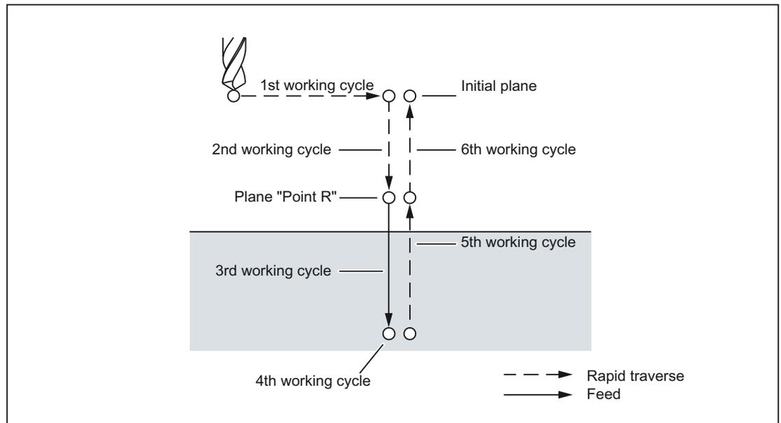
Figure 4-1 Sequence of operations in the drilling cycle
