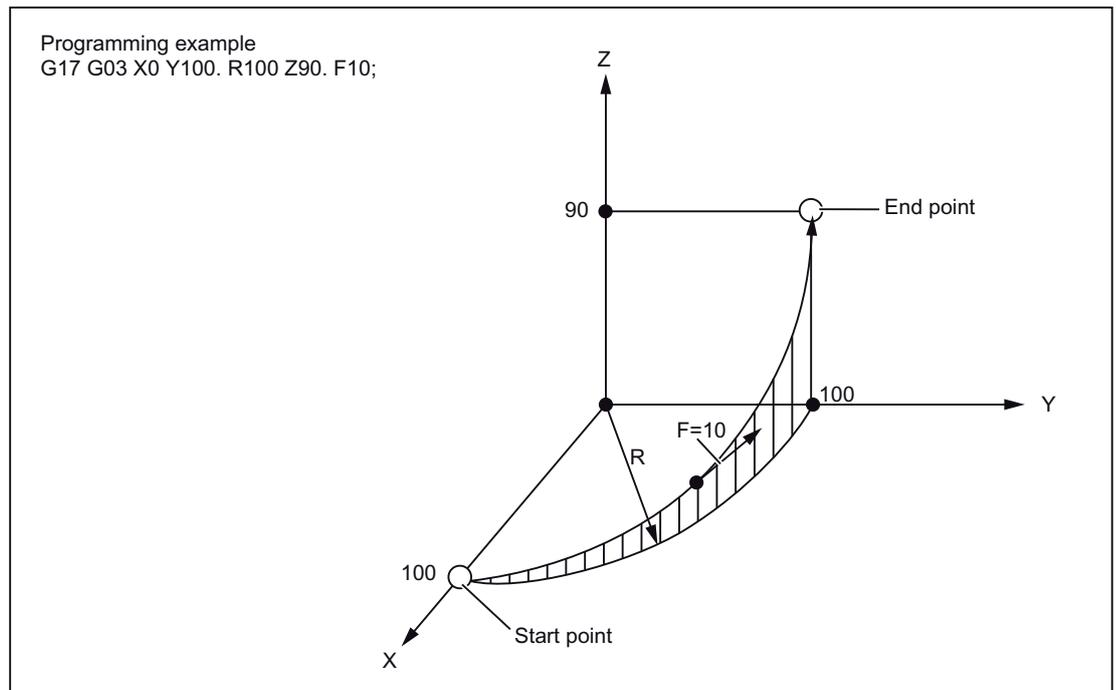
Figure 2-6 Helical interpolation
