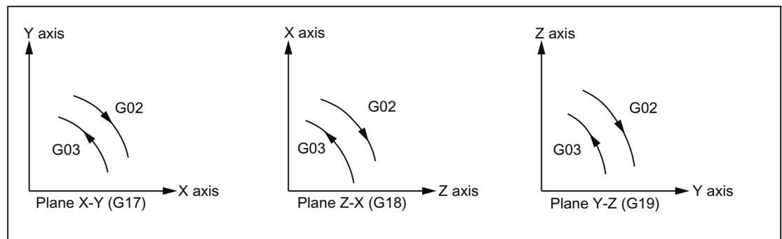
Figure 2-3 Direction of rotation of the circular arc
