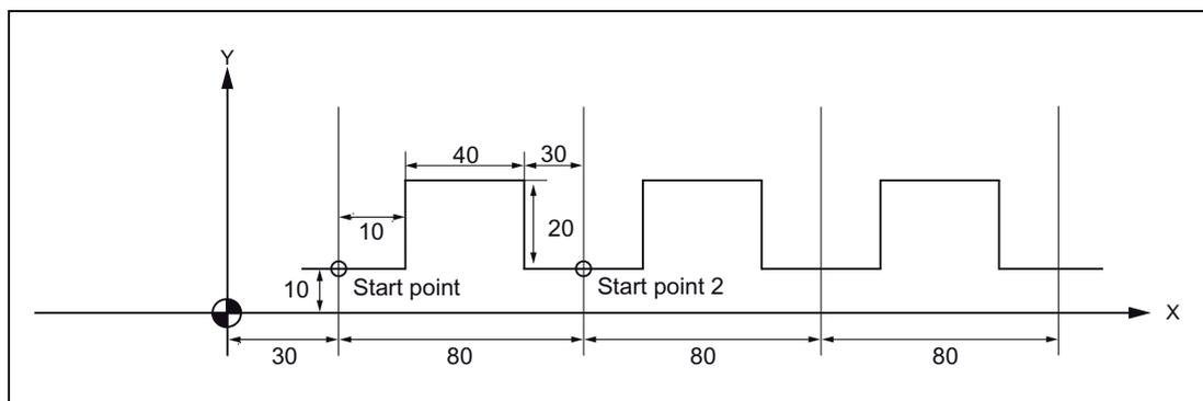
Figure 4-25 Contour repetition with G72.2
