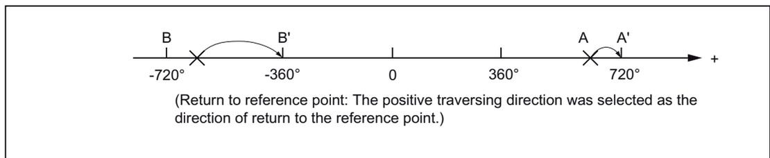
Figure 2-9 Return to reference point - rotary axes
