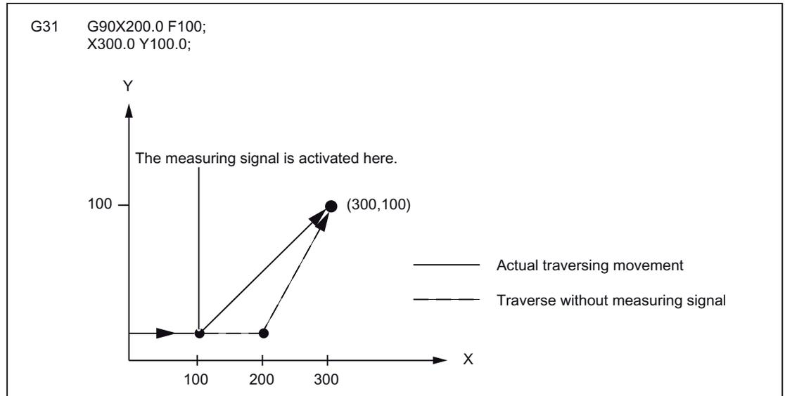
Figure 4-22 G31 is an absolute command for 2 axes
