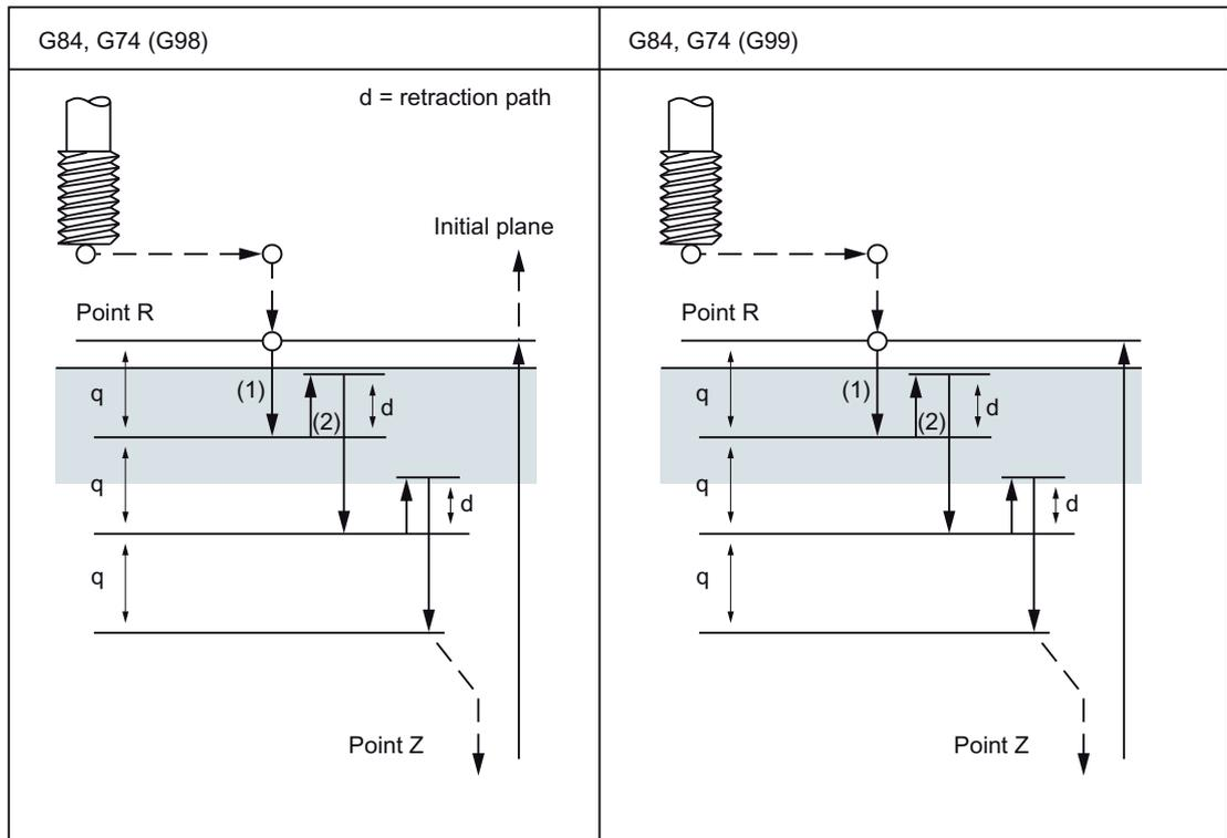
Figure 4-16 Deep-hole tapping with chip breakage (2)
