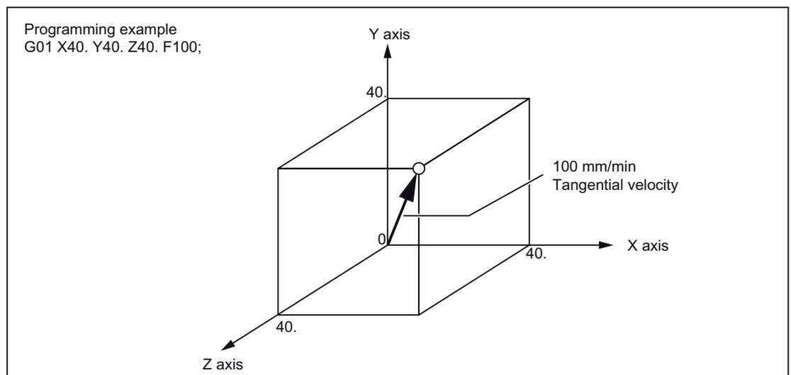
Figure 2-2 Linear interpolation
