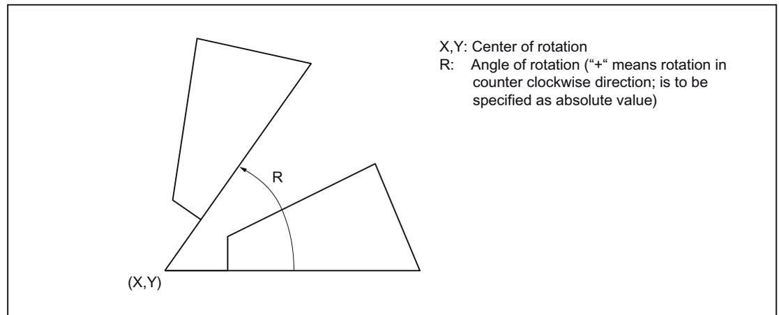
Figure 3-6 Rotation of a coordinate system
