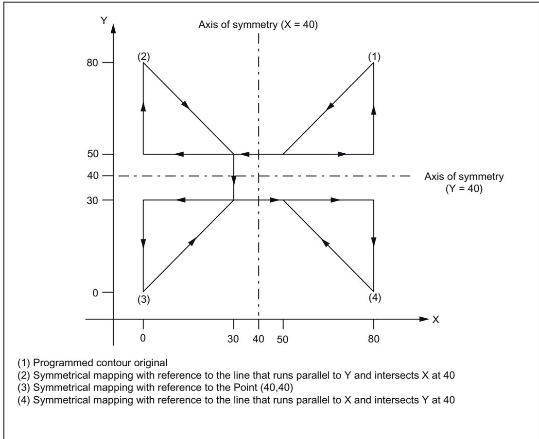
Figure 3-10 Programmable Mirroring
