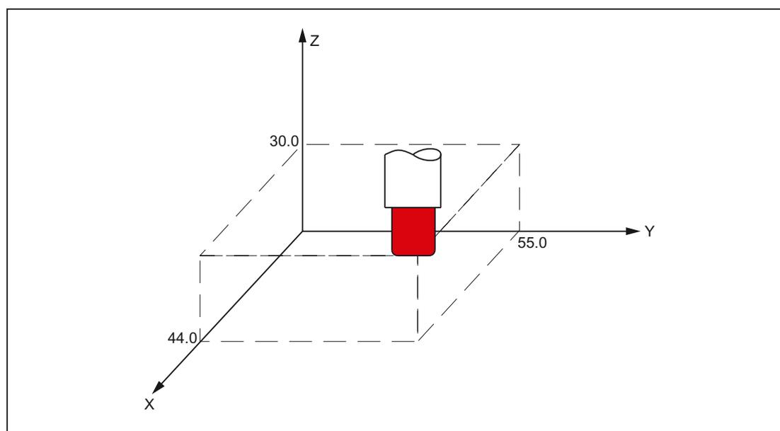
Figure 3-1 Tool positions specified with X... Y... Z...
