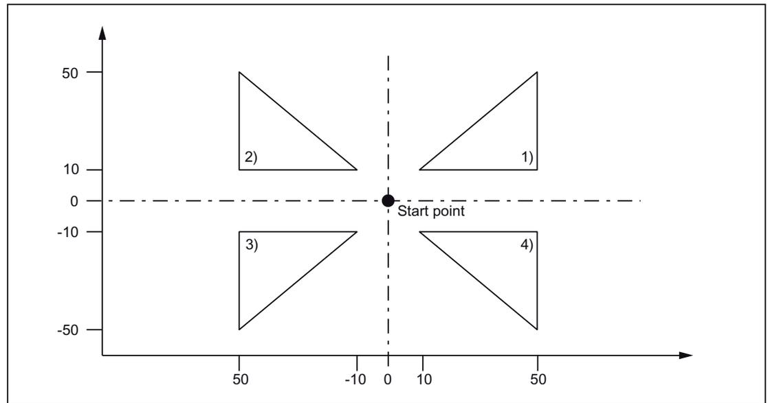
Figure 3-9 Scaling for each axis and programmable mirroring
