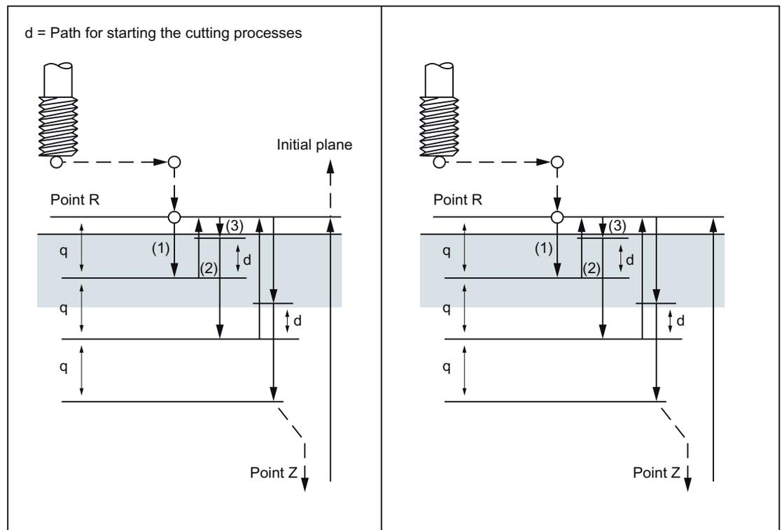
Figure 4-17 Deep-hole drilling with chip removal (3)
