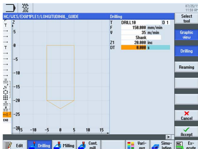
Figure 6-29 10mm drill holes
