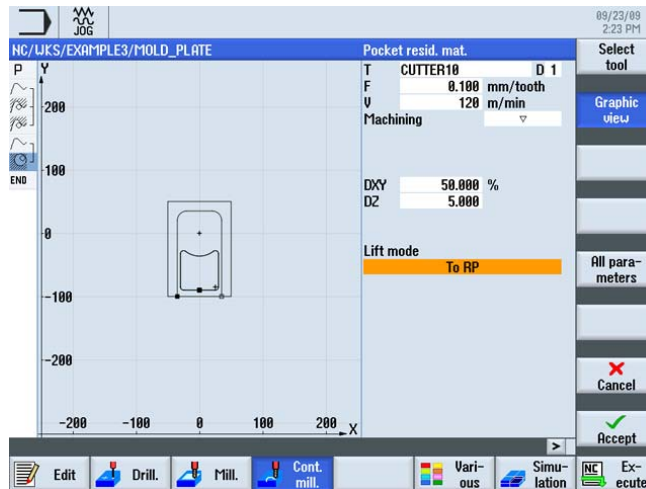
Figure 8-23 Machining residual material of the pocket
