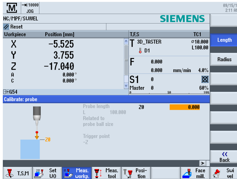
Figure 5-5 Calibrating the probe for the length
