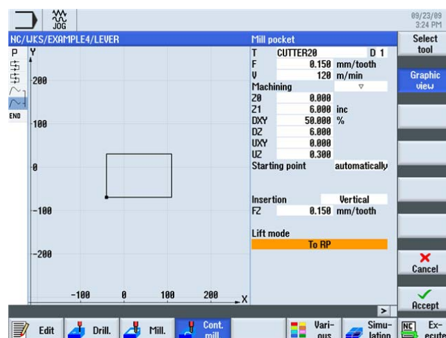
Figure 9-22 Roughing the contour
