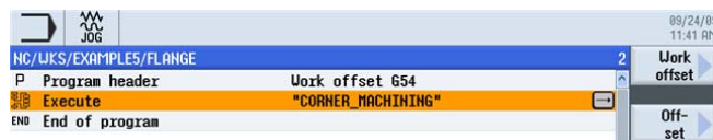
Figure 10-21 Subroutine pasted into the main program
