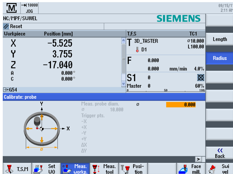
Figure 5-6 Calibrating the probe for the radius
