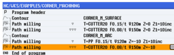
Figure 10-17 Complete subroutine in the work step editor
