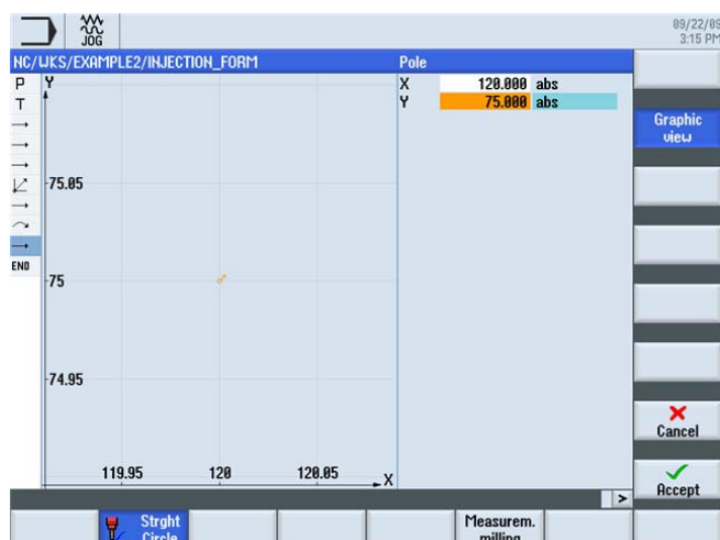
Figure 7-10 Specifying the pole for the circular path
