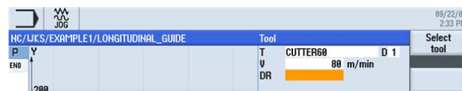
Figure 6-12 Tool cutting rate
