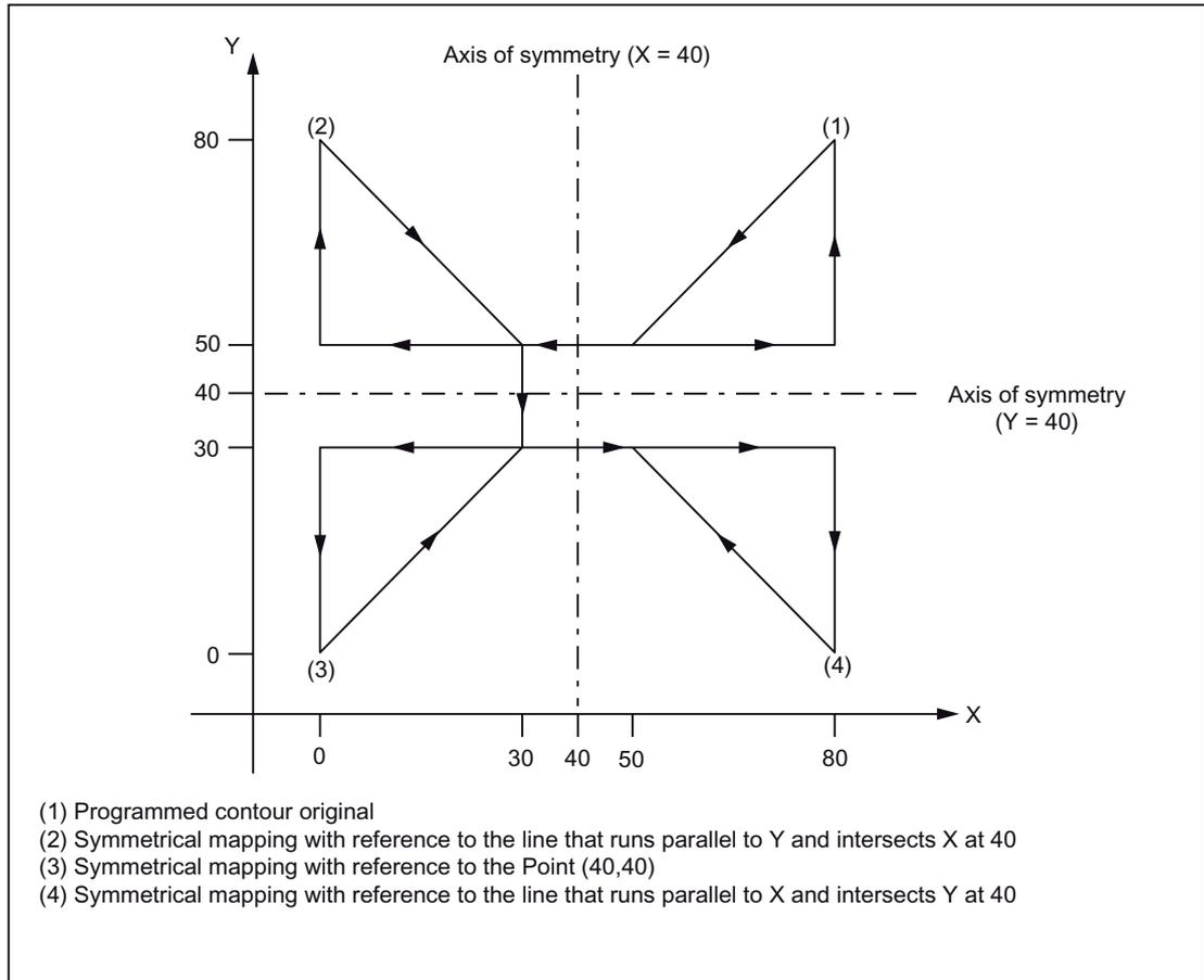
Figure 3-10 Programmable Mirroring
