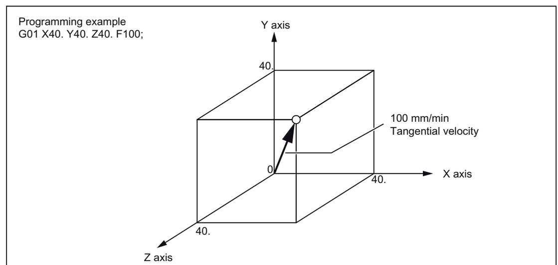
Figure 2-2 Linear interpolation
